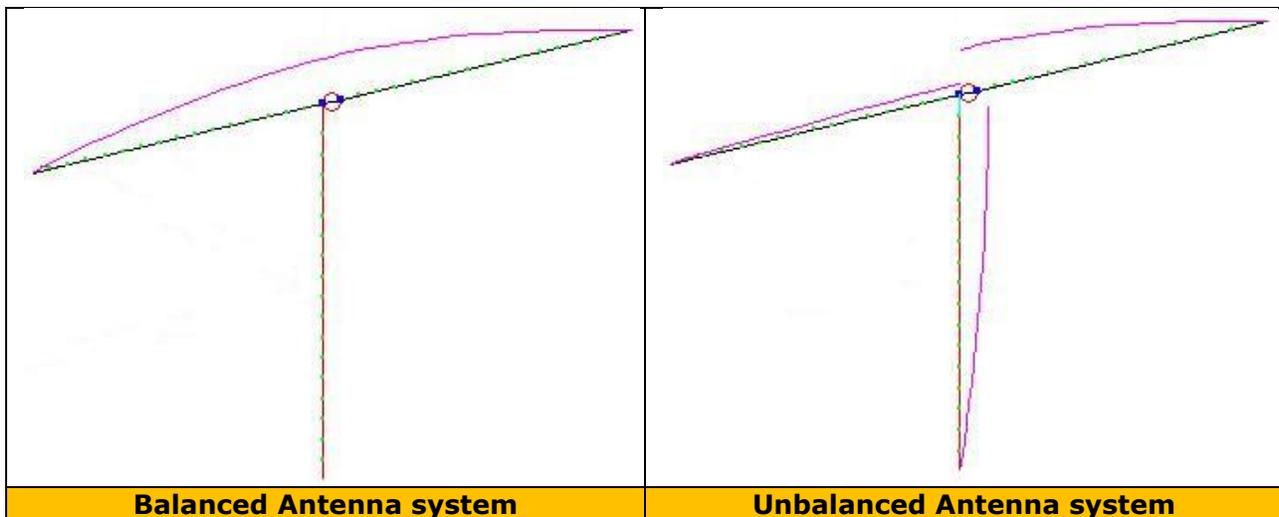
**Figure 4.** The currents on two dipoles: one with a balanced feed the other with an unbalanced feed. As can be noticed is that the current on one arm of the unbalanced system is significantly reduced, and instead, now a part of the current now on the transmission line itself. As a result the unbalanced antenna system will have worse radiation properties.
