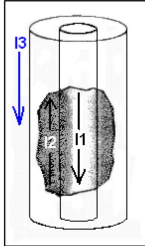
**Figure 2.** Currents on the inside of a coax cable (**I1** and **I2**) are equal and in opposite phase. Being **I1** the current on the inner conductor and **I2** the current on the inside of the cable shield due to the skin effect. But certain conditions may and shall induce or allow a current (**I3**) to flow on the outside of the coax cable shield.
