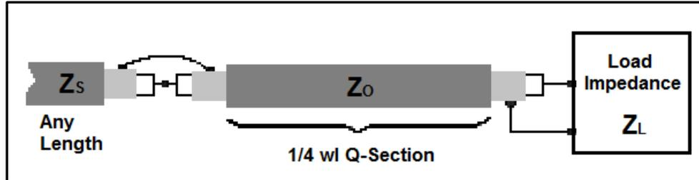
**Figure 11.8a.** A  $\frac{1}{4}$  wavelength Q Section impedance transformer.
