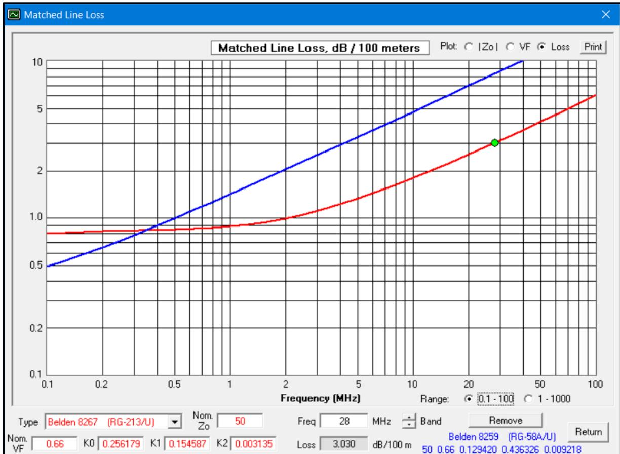
**Figure 11.5.** The Loss of either RG-58 or RG-213 coax cable for a length of 100 meters. Note at the top-right: a plot of the chosen transmission line characteristic impedance ( $Z_0$ ) and the Velocity Factor (VF), can also be displayed by checking its radio-button.
