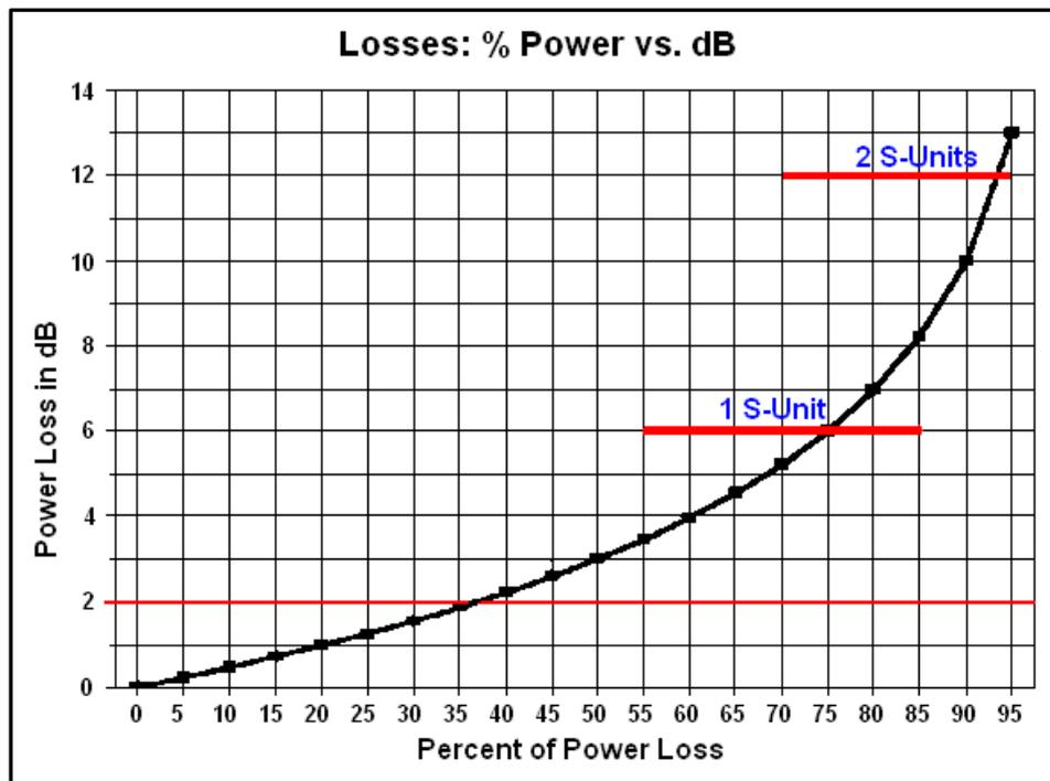
**Figure 11.6.** Percentage of power loss versus loss in dB and related S-Units
