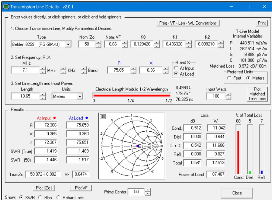
**Figure 11.7.** TLDetails program window. The top area shows the dialog boxes, at the bottom area the results.
