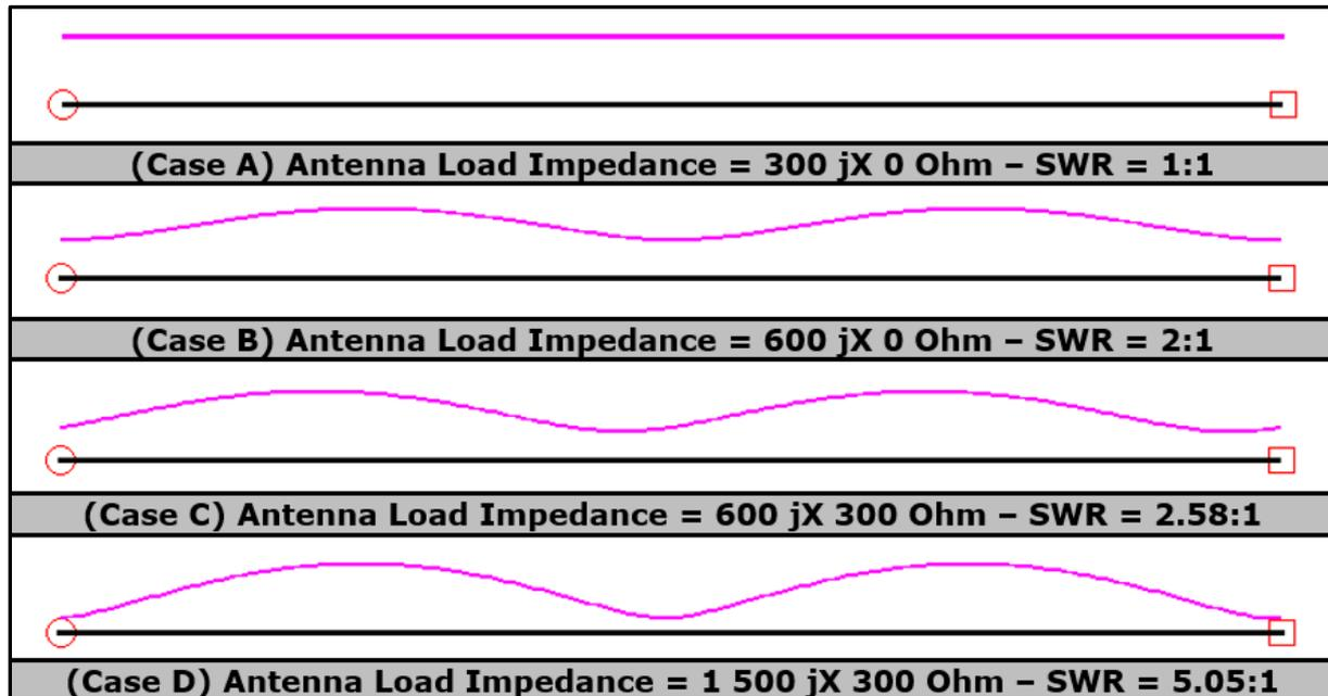
**Figure 11.4.** The current along a modeled transmission line with various antenna load impedances
