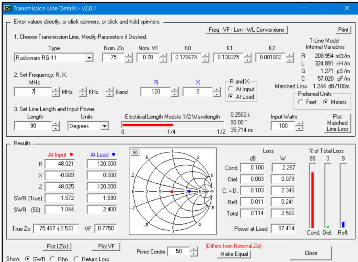
**Figure 11.8b.** Transforming an antenna load impedance of  $120\text{ j}X0\text{ ohm}$  to a 50-ohm coax (RG-213) and 50-ohm transmitter output, with a  $\frac{1}{4}$  wavelength (90 degrees) transformer section of 75-ohm characteristic impedance (RG-11). **Note:** compare the At Input data with the At Load data.
