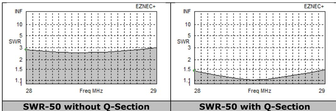
**Figure 9.8c.** Both SWR-50 plots of single quad loop: without or with 75-Ohm  $\frac{1}{4}$  wl Q-section.
