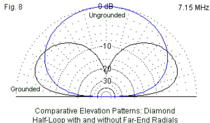
Although the low end-fed V may seem to be a reasonable NVIS antenna, it falls far short of the performance that we can obtain by raising the V to a top height between  $0.15 \lambda$  and  $0.2 \lambda$  above ground. Hence, the ungrounded version of the half-loop is not optimal for anything but emergency service--in which case, almost any wire that will radiate is suitable for service.
