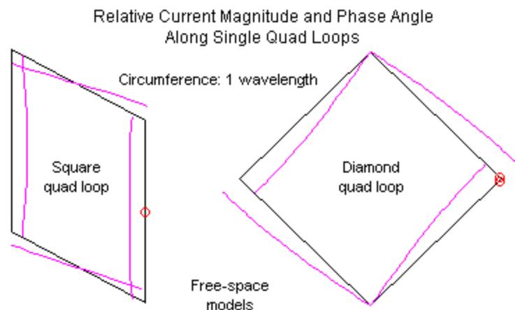
Essentially, then, the half-loop is one half of a quad loop, with the ground substituting for the missing lower half. A single quad loop has about 1.1 to 1.2 dB gain over a dipole, and over perfect ground, the half-loop has about 0.5-0.6 dB gain over a monopole. Unfortunately, unless we can construct a half-loop over an ocean (a good sea will do), we cannot obtain near-perfect-ground performance. Therefore, we shall have to satisfy ourselves with whatever the antenna will yield over dry ground.
