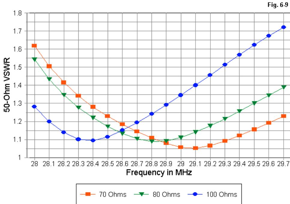
Although element diameter and phase-line  $Z_0$  produce relatively small changes in the performance curves compared to changing the length of the log-cell elements, these facets of log-cell Yagi design provide a measure of array design control. In effect, by varying one or both of these parameters, the designer can tailor the performance curves more closely to a desired profile.
