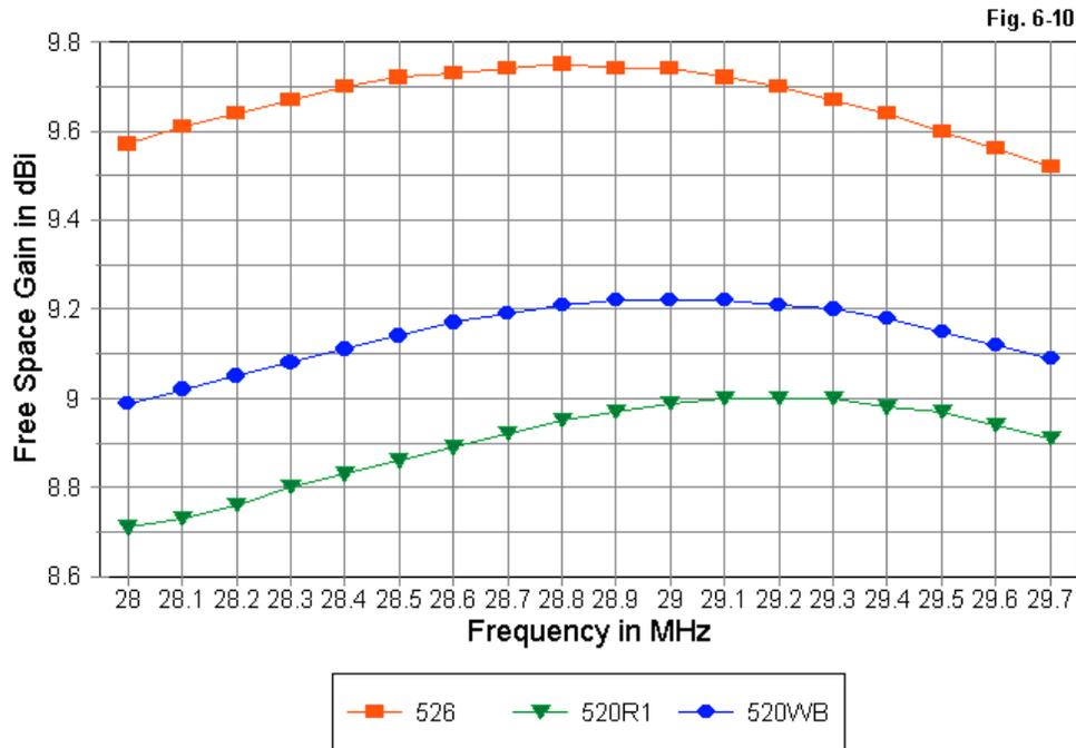
**Fig. 6-10** compares the gain of the three models on which we are focused. 526 has the highest and best-centered gain curve. However, the wide-band version of 520 shows increased gain and better curve centering relative to the design version on which it is based. Part of the
