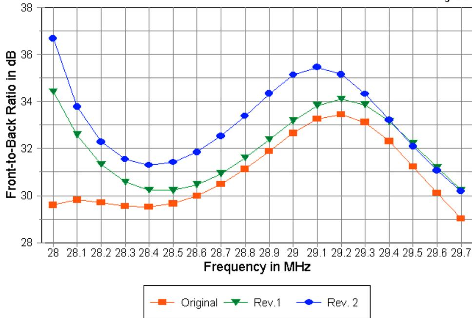
Higher peak gain also results in a somewhat lower front-to-back value across the band, as revealed in **Fig. 6-2**. Changing the log-cell element length to smooth out the gain actually produces greater variations in the front-to-back ratio across the band. One conclusion we may reach from these curves is that the smooth front-to-back curve in model 526 does not result alone from centering the gain curve by lengthening log-cell elements.
