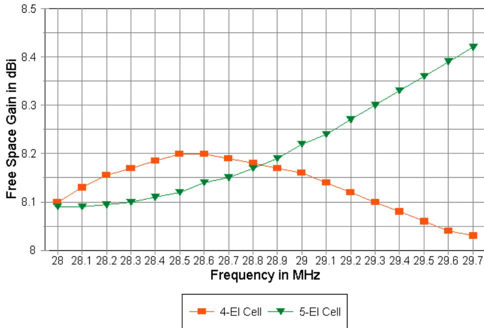
As shown in **Fig. 5-3**, the gain curves for the two antennas differ in form—a factor that will become one of the design questions to be explored. The initial values of the 5-element cell array are lower than those of the 4-element cell array, although the larger array shows a steady increase in gain across 10 meters.
