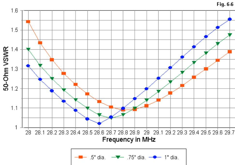
In every respect, the effects of increasing the element diameter in a log-cell Yagi can be classified as normal to the LPDA behavior of the log cell.
