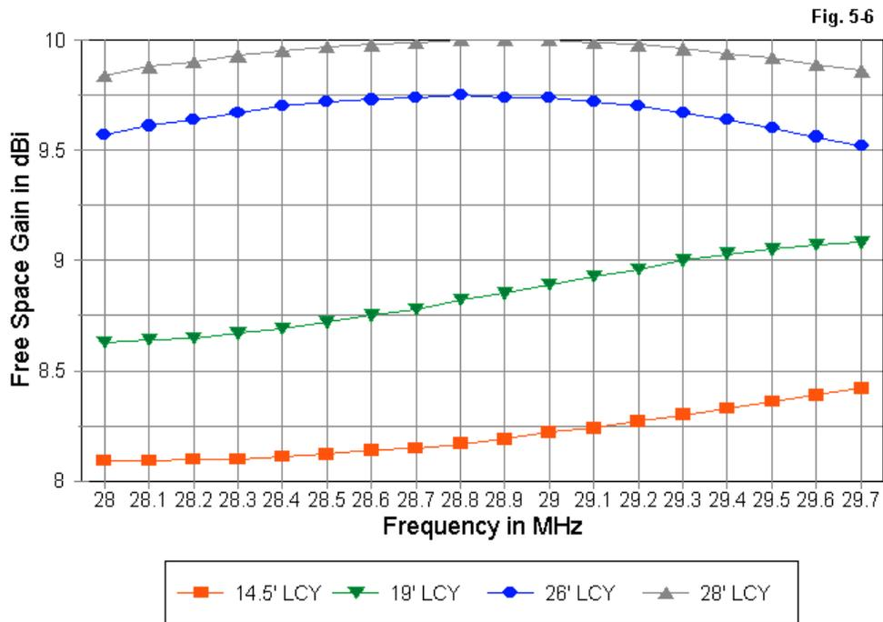
**Fig. 5-6** shows the free-space gain curves for models 514 through 528. On the wide-range gain scale, the upward progression of gain in 514 is put into somewhat better perspective to display the 0.33 dB total gain change across the band. Model 520 is about 4.5' longer overall and displays a similar gain curve. However, the upper end of the curve is reaching its peak value as the rate of increase approaches zero.
