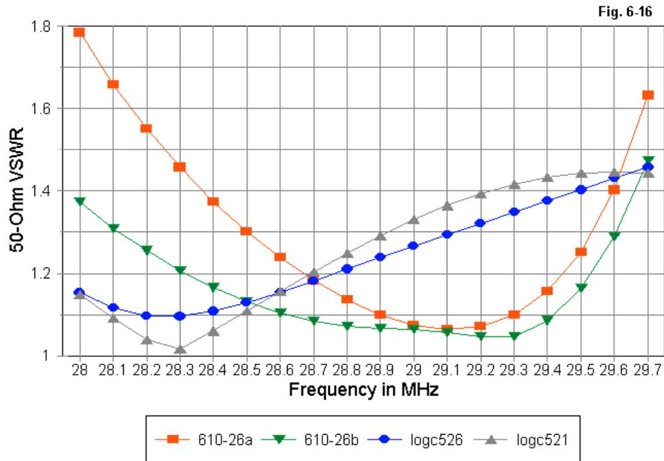
The comparison of the long-boom Yagi to the long-boom log-cell Yagi is designed solely to place a few specifications in perspective. Consistent with the results for short-boom log-cell Yagis, long-boom log-cell Yagis do not yield as much forward gain as comparably long pure Yagi designs. However, the log-cell Yagi can be tailored to yield either very high front-to-back values or to have roughly equal gain and front-to-back values across a band as wide as 10 meters.
