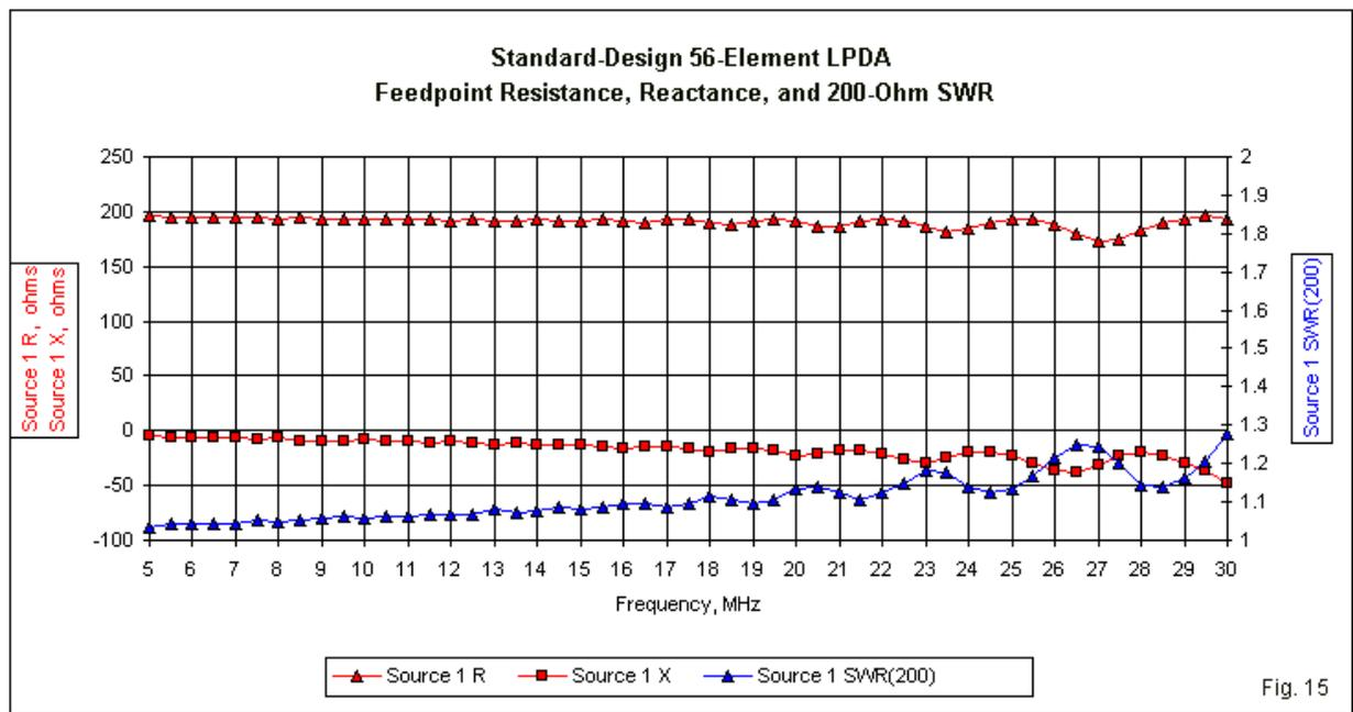
The standard 56-element LPDA shows equal control of the feedpoint properties across the operating range in **Fig. 15**. As the frequency increases and the number of forward elements become less numerous, the curves show an increasing level of undulation. However, the 200- $\Omega$  SWR does not reach 1.3:1 by 30 MHz.
