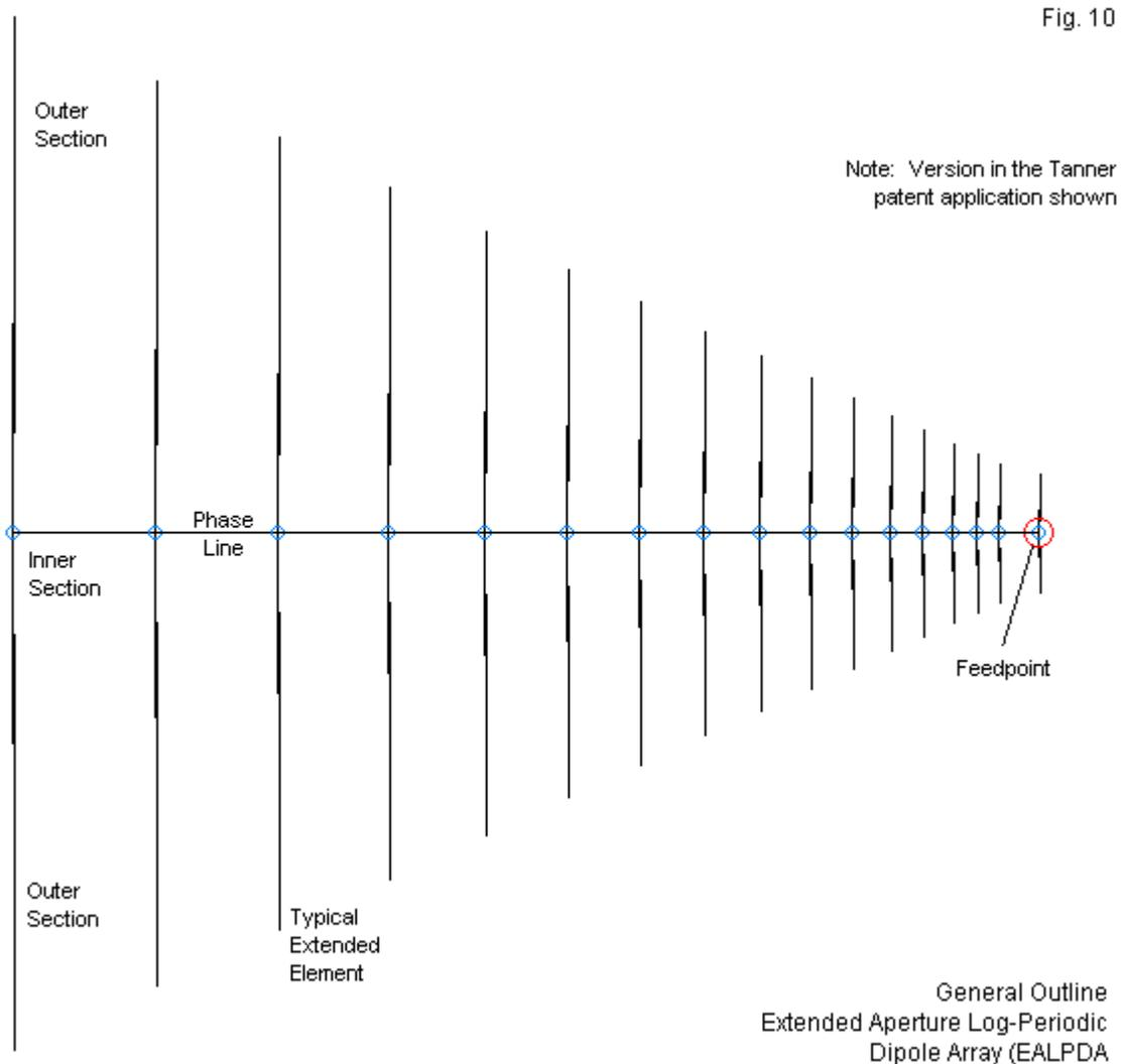
The applicable value of  $\tau$  for the EALPDA is 0.875, well below the 0.96 value of  $\tau$  necessary to achieve the performance of the standard LPDA. For a  $\tau$  of 0.875, the standard equation gives an optimal  $\sigma$  value of 0.161, but the patent design has a  $\sigma$  of about 0.170. In addition, the
