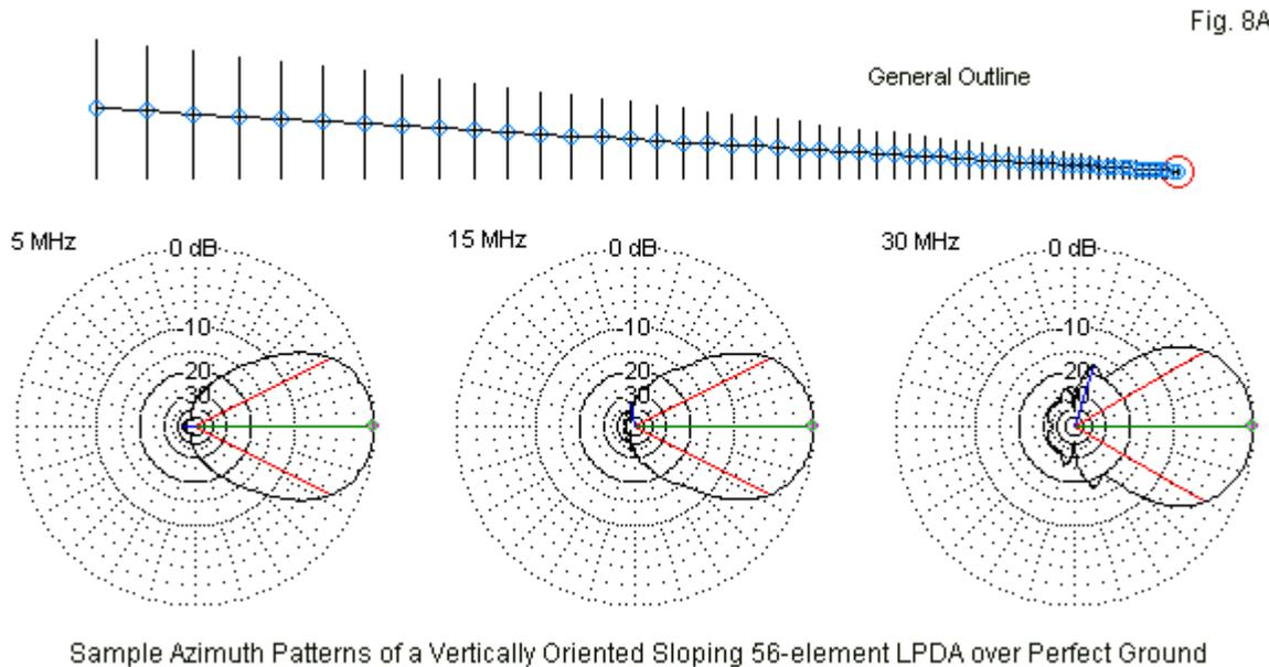
**Table 7** contains the results of the modeling exercise over perfect ground and then over three real ground qualities: very good, average, and very poor. The table shows us the sort of performance changes that a vertical array may undergo with changes in the soil quality beneath the array.
