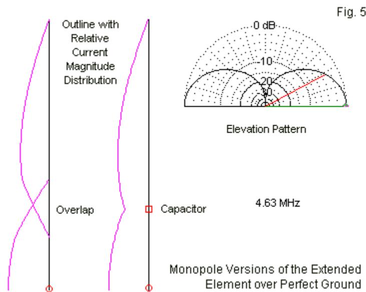
**Table 2** lists the essential properties of the extended elements as monopoles, along with information on a reference  $\frac{1}{4}\lambda$  monopole at the design frequency. Each antenna is exactly half the length of its dipole counterpart. The extended elements are 100' long. The capacitor position is 30' above perfect ground. The overlap extends from 19.5' to 40.5'. The monopole is 51.6' long. All use the standard lossless 0.16"-diameter wire.
