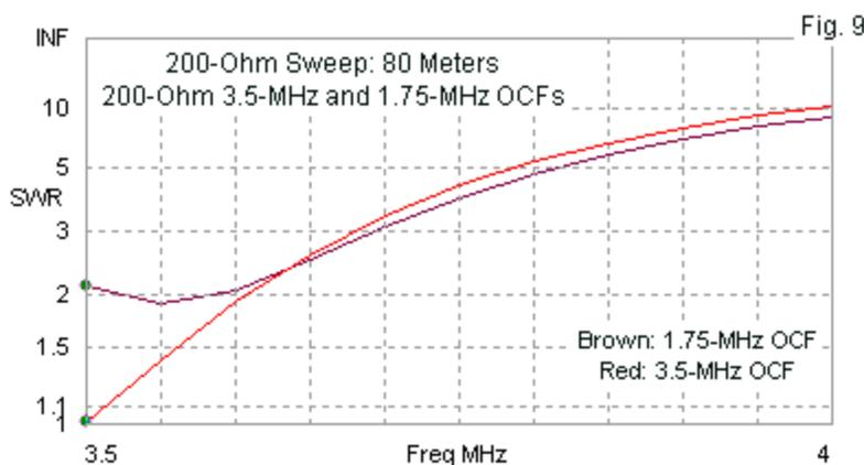
The use of free-space SWR sweeps is subject to modification when we place the antenna over real ground at a fixed height. 50' is only about  $0.2\lambda$  above ground on 80 meters, a region in which we may find large swings of feedpoint impedance in a fixed-length antenna for relatively small changes in antenna height. Any decisions in this matter would have to rest upon more detailed analyses tailored to the height at which a user proposes to install the antenna.
