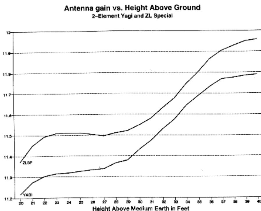
Fig. 7. Yagi and ZL Special gain vs. height above ground from 20' to 40' over real medium earth.
