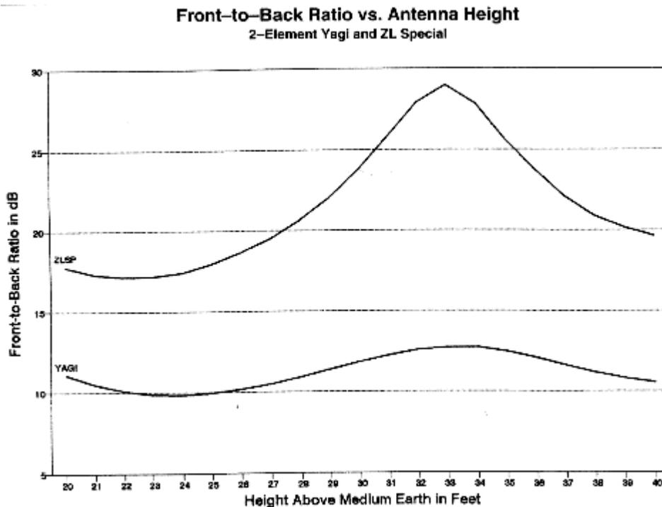
Fig. 8. Yagi and ZL Special front-to-back ratio vs. height above ground from 20' to 40' over real medium earth.
