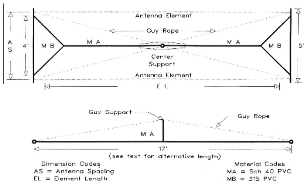
Fig. 9. General sketch of a single-mast support structure for testing wire ZL Specials.
