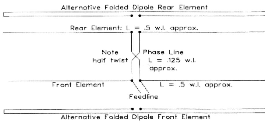
Fig. 1. The basic construction of a ZL Special horizontal 2-element phased array.
