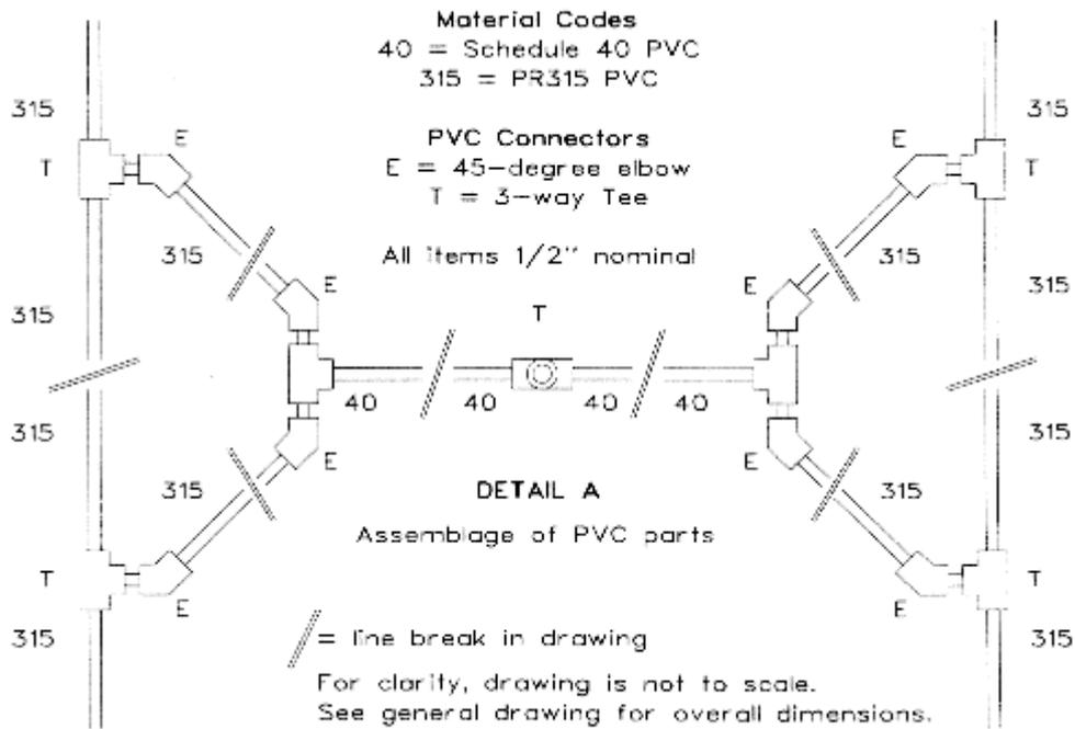
Fig. 10. Detail A of the support structure, showing the combination of PVC materials used in its construction.
