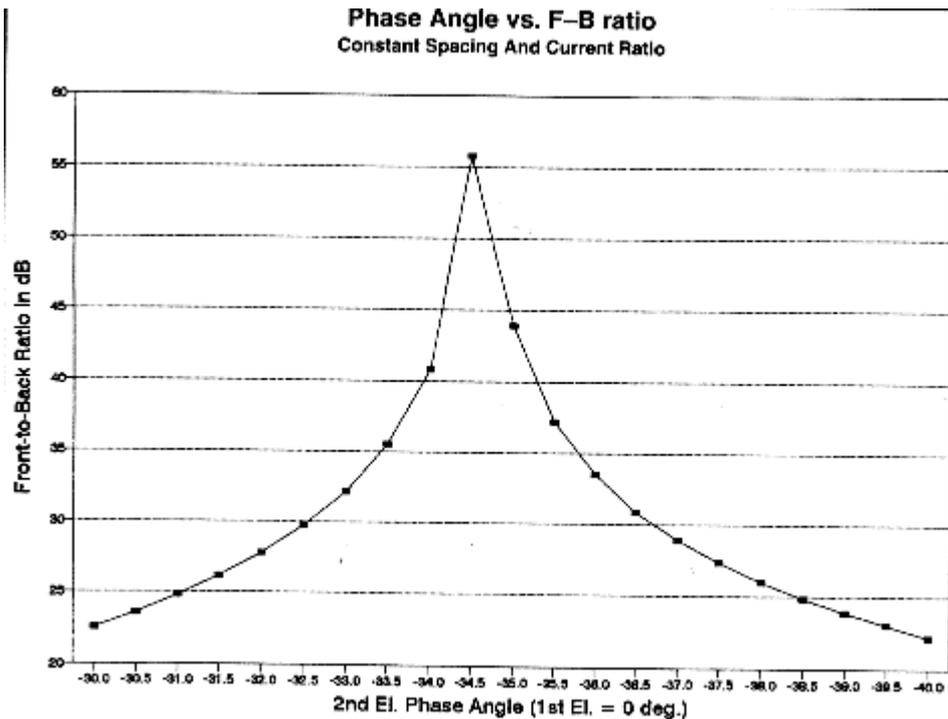
Fig. 4. Front-to-back ratio vs. phase angle for two-element arrays.
