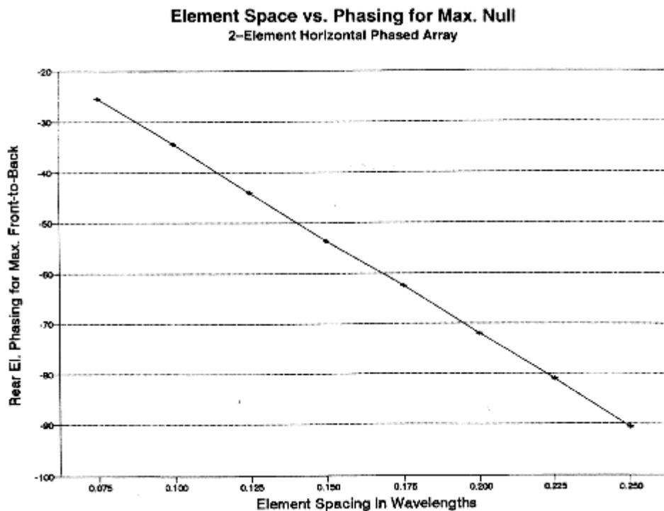
Fig. 3. Graphic representation of the relationship between ZL Special element spacing and the phase angle required for maximum front-to-back ratio.
