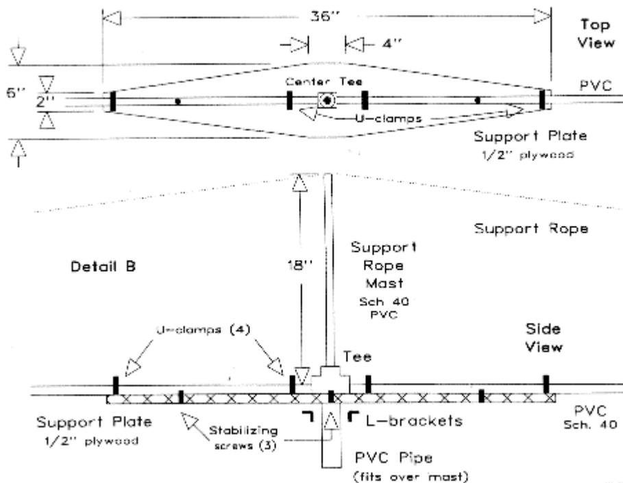
Fig. 11. Detail B of the support structure, showing the center plate and mast connection.
