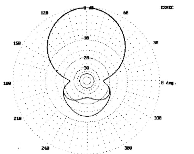
Fig. 2. Comparison of azimuth plots for the reference Yagi and a ZL Special at 28.5 MHz, 35' above real medium earth.
