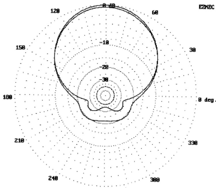
Fig. 13. Azimuth patterns of the 'BRD Zapper at 28.5 MHz, 20' and 35' over real medium earth.
