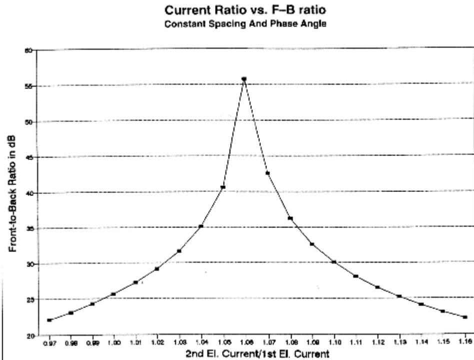
Fig. 5. Front-to-back ratio vs. current ratio at element feedpoints for two-element arrays.
