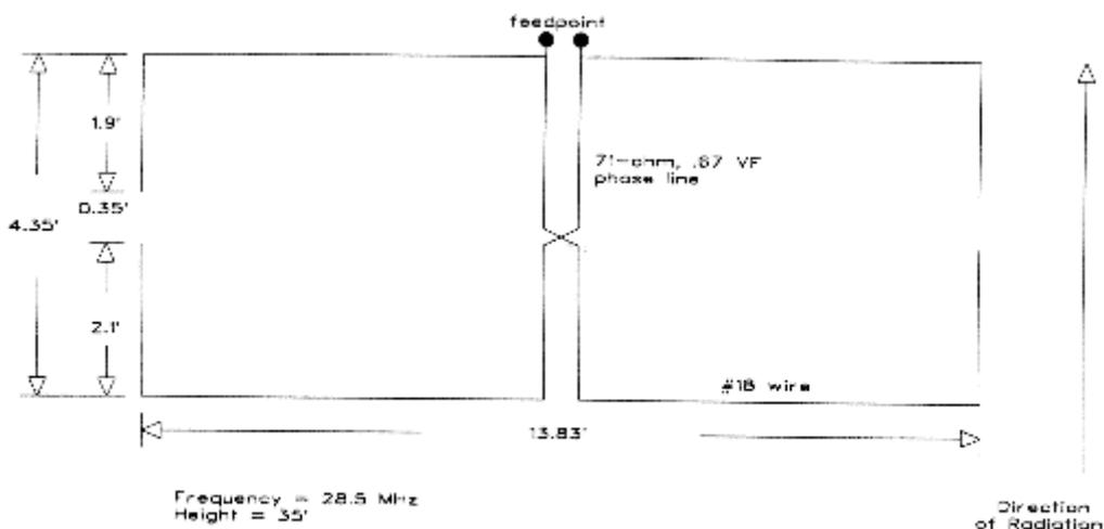
Fig. 12. General configuration of the 'BRD Zapper ZL Special.
