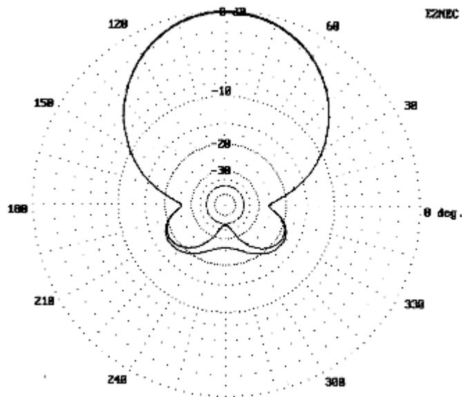
Fig. 6. Comparative azimuth patterns for equal-length element and "improved" versions of the 5/8" straight dipole ZL Special (35' above real medium earth).
