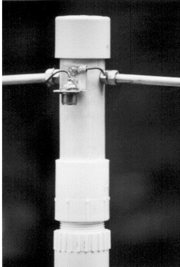
8 A close-up of a PVC dipole element hub for aluminum rod elements.
