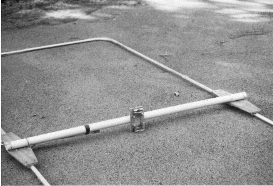
6 A Moxon rectangle using a PVC boom with element and boom plates.
