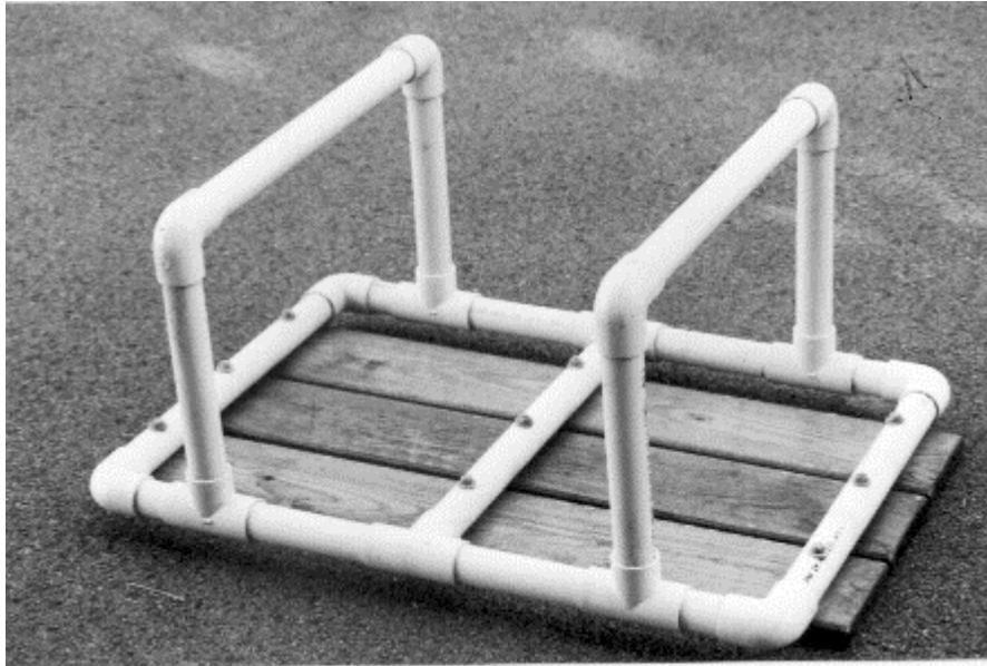
2 A bottom view of a yard bench illustrating some PVC assembly techniques.
