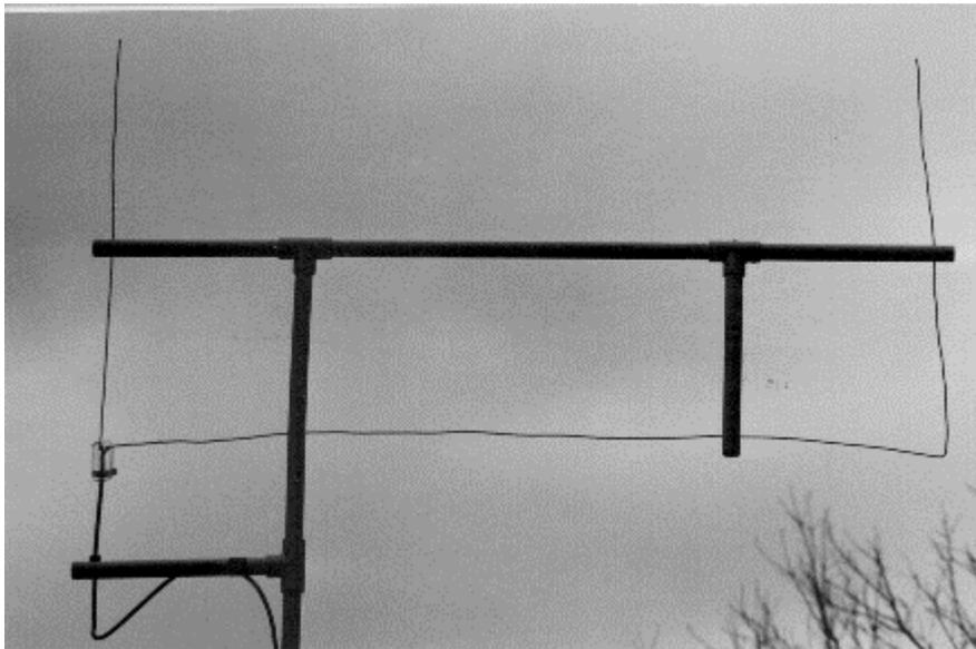
10 A #12 AWG wire 2-meter half square on a PVC test frame.
