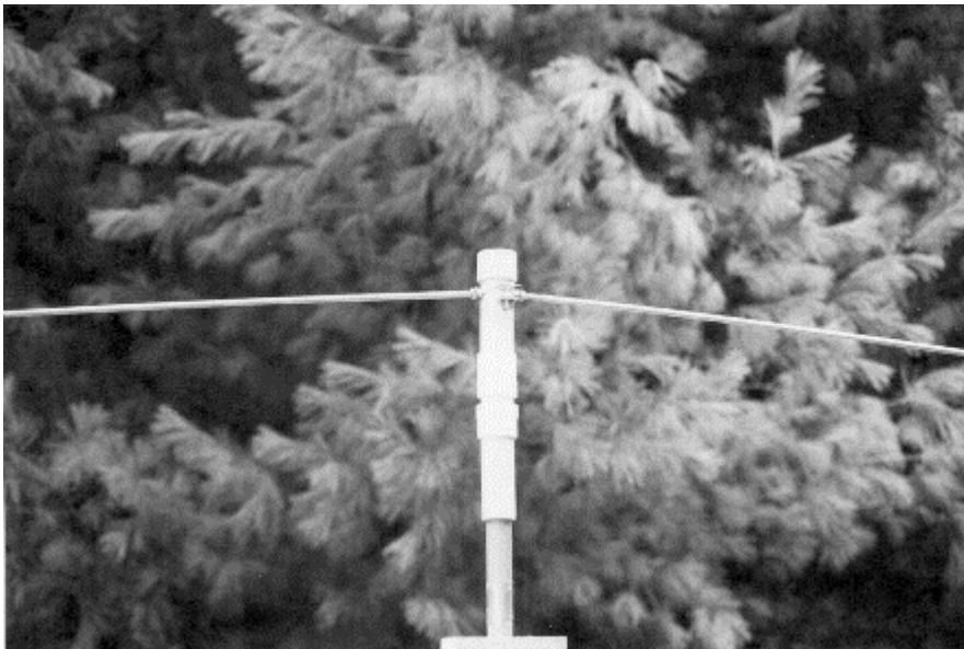
7 A portable dipole with a PVC hub and screw fitting, mounted on a steel mast.
