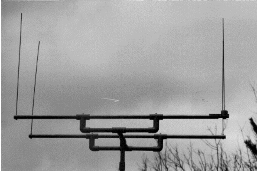
11 A more complex PVC mounting frame for a 2-element 2-meter half-square beam.
