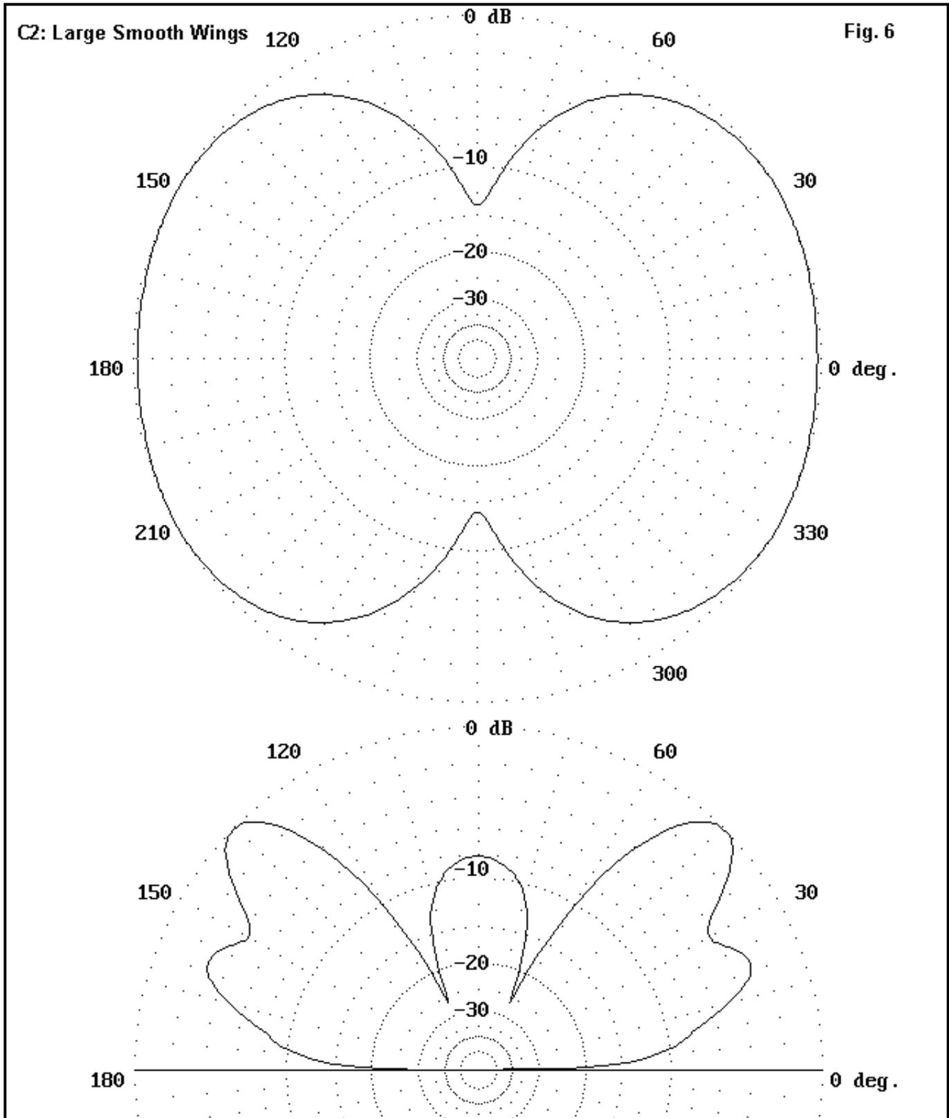
Large smooth wings, shown in **Fig. 6**, develop as we change the loop shape or increase the frequency somewhat further. Notice that now the radiation is off the edges of the loop and is no longer broadside to it. In addition, the elevation pattern is marked by multiple lobes. For any given case, either the lower or the upper lobe may be stronger--or they may both be at about the same
