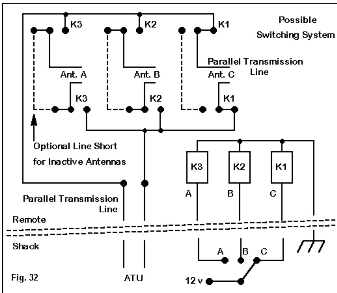
**Fig. 32** shows one possible switching system for remotely controlling which antenna is active. The in-shack controller can use almost any indicator system the user might imagine. Therefore, I shall leave further refinements to the reader's sketch pad.
