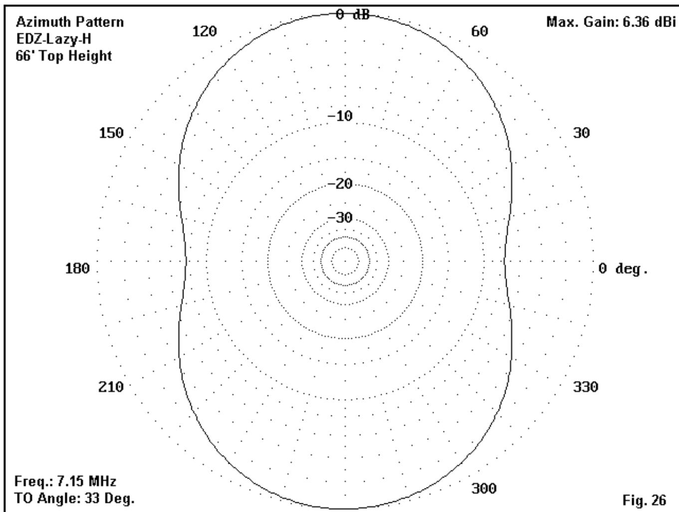
On the lowest band of operation, 40 meters (**Fig. 26**), the pattern has become an oval, with just a trace of the peanut shape. As we earlier noted, the gain is less than that of the single 10-meter EDZ or the 67' doublet, but it is still high enough to provide excellent coverage.
