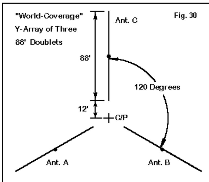
**Fig. 30** shows one way to accomplish the desired goal. If we have the room and the supports--in short, if we live in a forest--we can set three Lazy-H arrays in a Y pattern. The sketch shows the larger version, but you can always directly scale the dimensions for the smaller 40-10 meter version.
