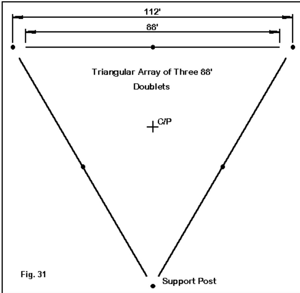
A standard triangle (**Fig. 31**) offers a more compact arrangement of the antennas and needs only three supports--just one more than a single Lazy-H would require. Once more, scale the space down for the smaller array. As with the Y, variations in the exact angles of each array will not be noticed except in the better aim we obtain for each Lazy-H relative to our communications targets.
