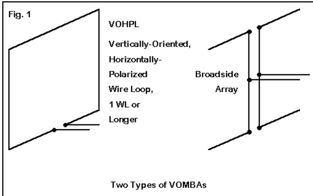
**Fig. 1** also shows a second vertically oriented array: the Lazy-H. One of a number of in-phase-fed arrays, the Lazy-H is also horizontally polarized. In traditional terms, this is a broadside array, since radiation is strongest perpendicular to the plane defined by the two radiating wires. (In contrast, a Yagi is an end-fire array, since radiation is in the plane of the elements.)
