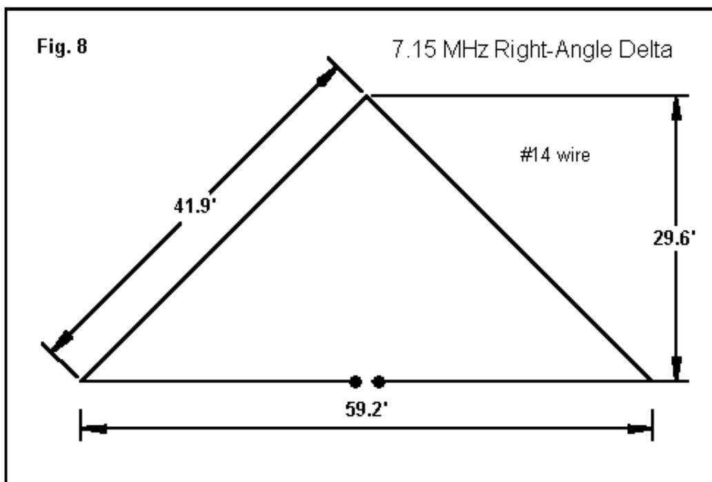
The right-angle delta appears in **Fig. 8**. With a top height of 66', it has a lower horizontal wire at about 36.6' up. In the table following the sketch of the right-angle delta, the lowest angle data are shown if the lowest lobe is either dominant or if it is close to equalling a higher more dominant lobe.
