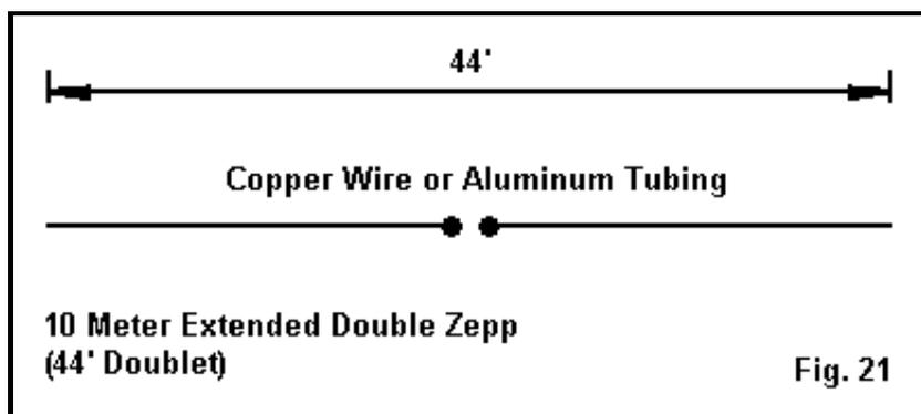
Notice that the sketch bears a second name for the antenna: the 10-meter extended double Zepp or EDZ. On 10 meters, the antenna is about 1.25 wl long, the standard EDZ length. On 15 meters, the antenna is just about 1 wl long. On 30 meters, it is just a bit short of a 1/2 wl dipole. On 40 meters, the antenna is in the vicinity of 3/8 wl long.
