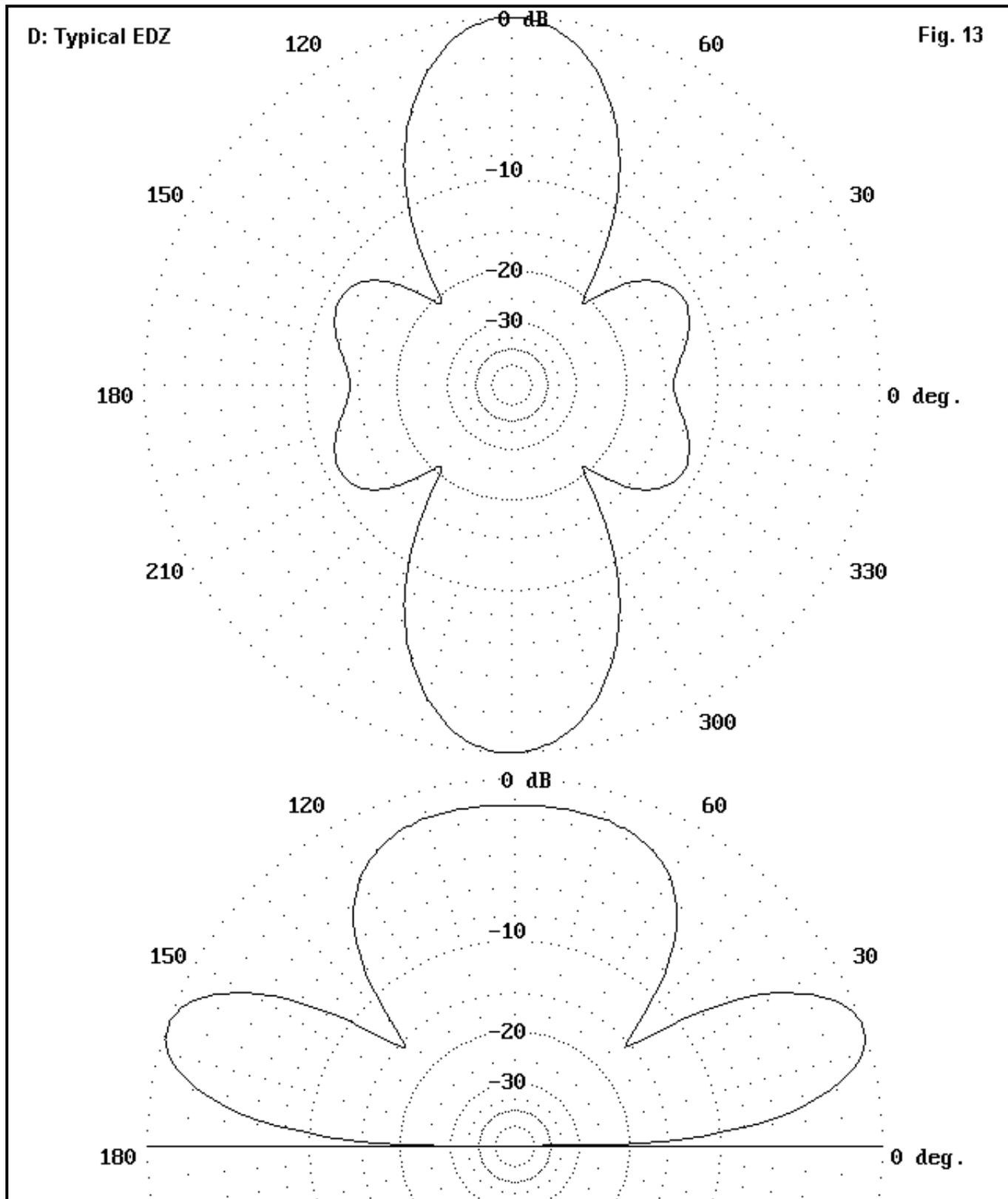
**Fig. 13** shows a typical set of azimuth and elevation patterns for an extended double Zepp--or EDZ. On 17 meters, the 40-meter doublet is about 1.25 wl long and hence exhibits these patterns. The azimuth pattern main lobe is considerably narrowed relative to our typical peanuts (A2), and new lobes are beginning to show up as a set of "ears" on the azimuth pattern. However, the
