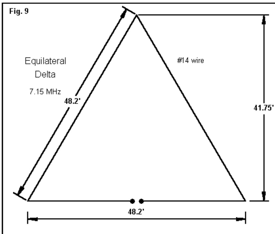
An equilateral delta (**Fig. 9**) is taller but narrower than its right-angle cousin. With a 66' top, the equilateral delta is about 12' closer to the ground at the bottom. This makes a difference in the performance, especially above 40 meters.
