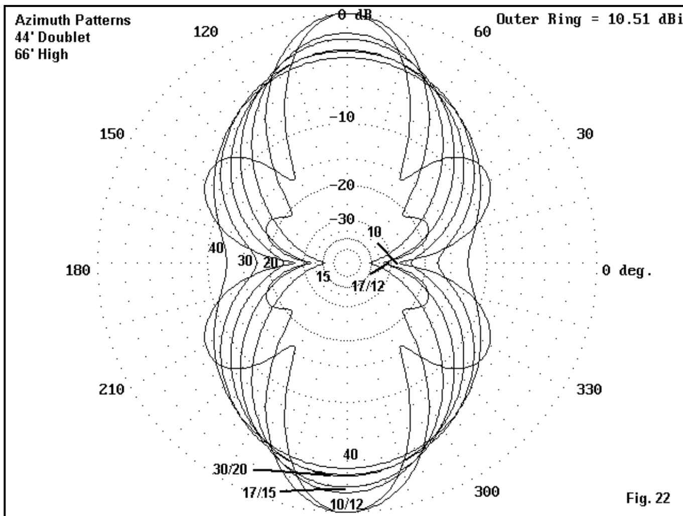
By setting the maximum length of the doublet at the 1.25-wl mark on the highest frequency we plan to use, we obtain bi-directional patterns for all of the bands (40 through 10 meters). The same principle can be applied for any 4:1 frequency ratio: for example, an 88' EDZ/doublet to cover 80
