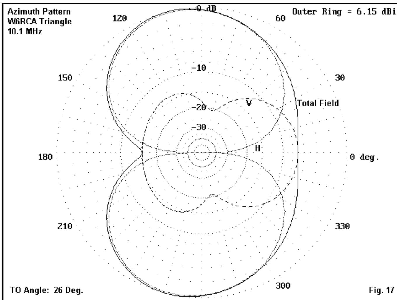
**Fig. 17** shows the azimuth pattern of the triangle on 10.1 MHz, where the TO angle is 26 degrees. In general, the pattern qualifies as an A pattern, but with a difference. The left side is a peanut, while the right side is an oval, giving us a kidney bean. The feedpoint and the vertical leg of the triangle are at the right, as shown in the sketch in **Fig. 16**. The antenna is 30' above ground, for a top-wire height of 60'.
