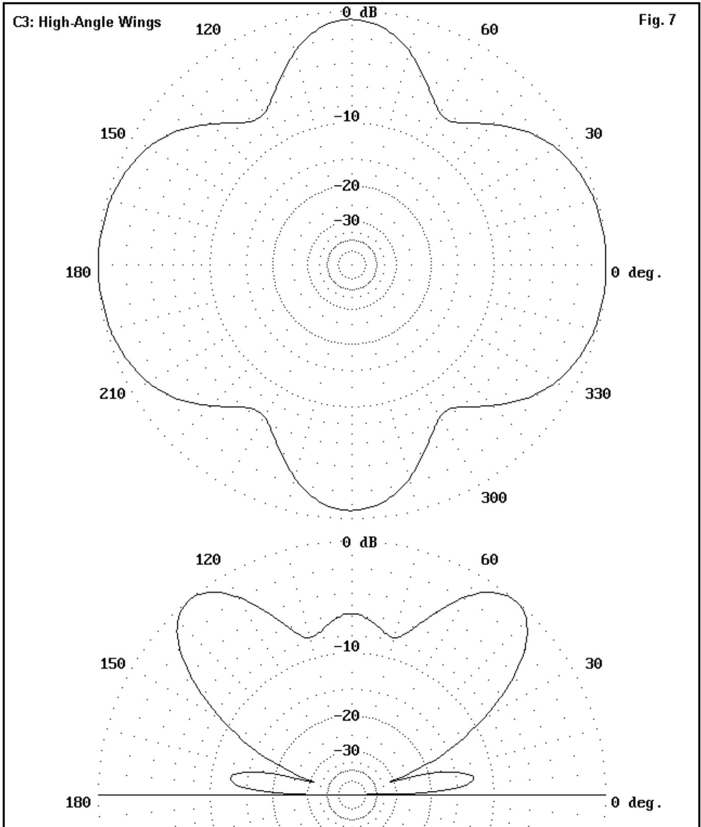
Sometimes, the development of side-wings in the azimuth pattern is accompanied by an almost complete loss of low-angle radiation. **Fig. 7** shows the patterns for such a case, which is common on the upper HF bands for some 40-meter loops. Although the azimuth pattern may show a high gain figure, the gain is often at angles too high in the upper HF region to do more than bring in an
