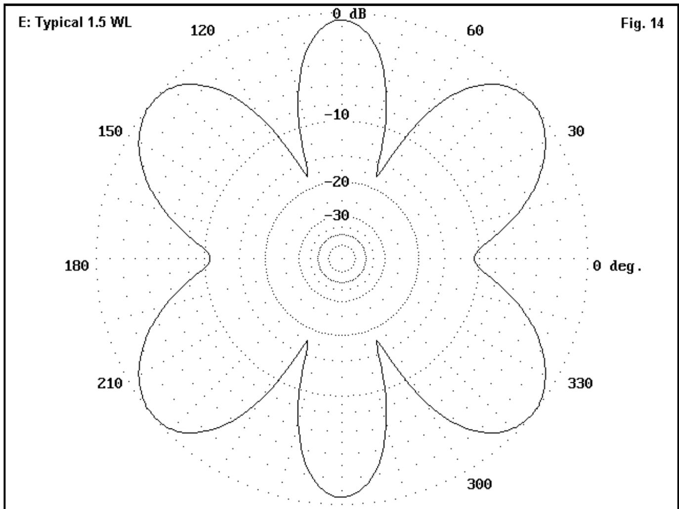
When the antenna is about 1.5 wl long, the 6-petal pattern of **Fig. 14** emerges. Here, we have radiation lobes of roughly equal strength in 6 different direction. This is the 40-meter doublet pattern on 15 meters. Since the elevation patterns of the doublet are so well-behaved, I have omitted them in these figures.
