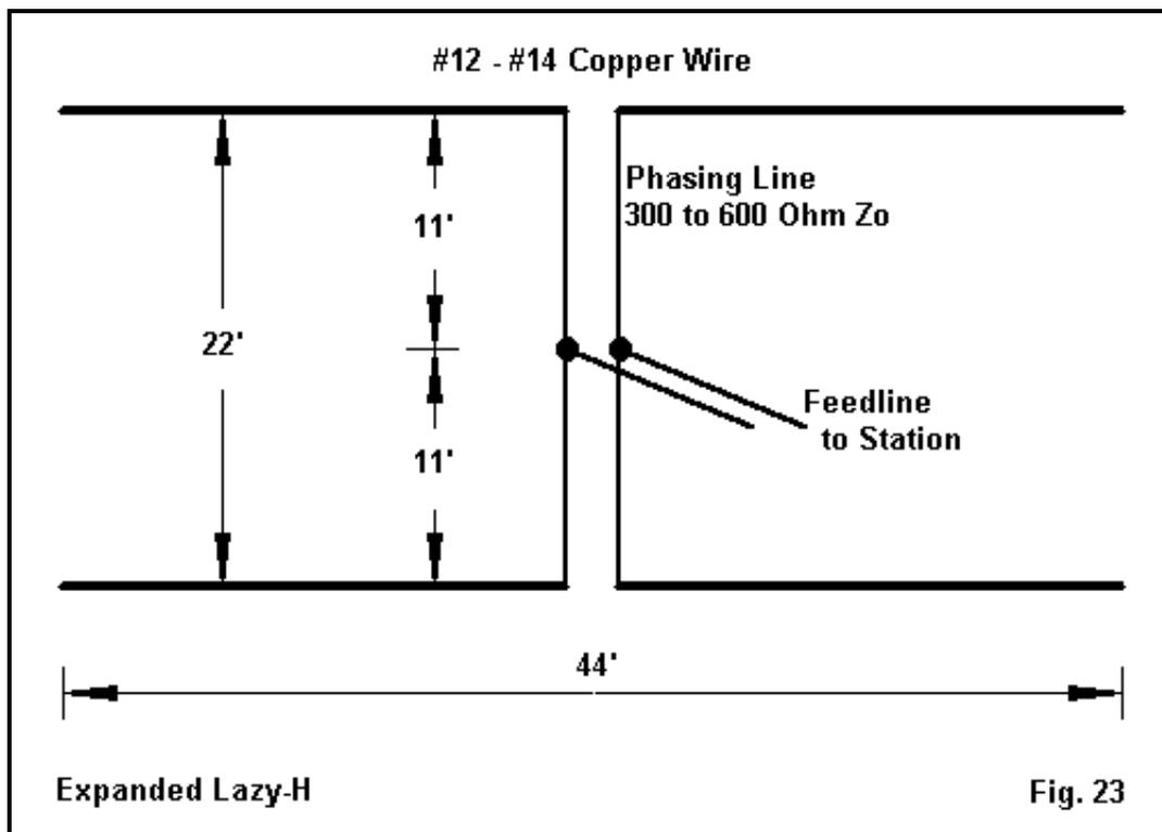
We have some options in how we think about the expanded Lazy-H for 10 meters. Actually, the antenna is a standard 1-wl by 1/2-wl Lazy-H for 15 meters. Alternatively, it is an array of 2 10-meter EDZs, each 44' long. However, we think about the antenna, the spacing is 22', so if we place the top wire at 66' up, the bottom wire is at the 44' mark. If we have the ability to put up a 44' wire doublet, the odds are that we can also construct an expanded Lazy-H.
