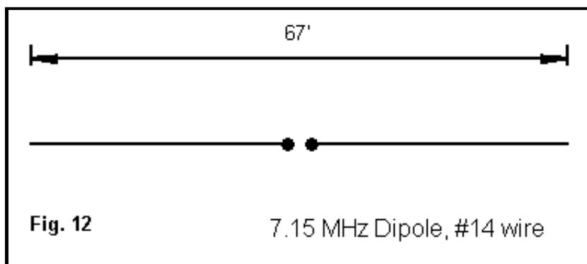
A 67' doublet is approximately resonant on 40 meters (**Fig. 12**). At a height of 66', it is also about a half wavelength up, which is a reasonably good height for dipole performance. Above 40 meters, the antenna become a doublet for open wire transmission line and ATU use. As the table shows, it acquits itself quite well.
