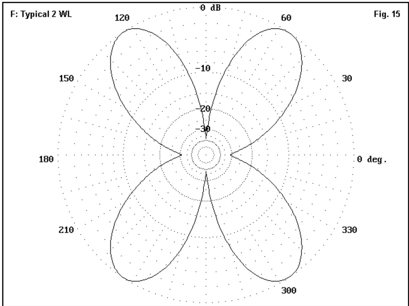
On 10 meters, the 40-meter doublet is 2 wl long. Its azimuth pattern, as shown in **Fig. 15**, becomes as 4-petal affair.
