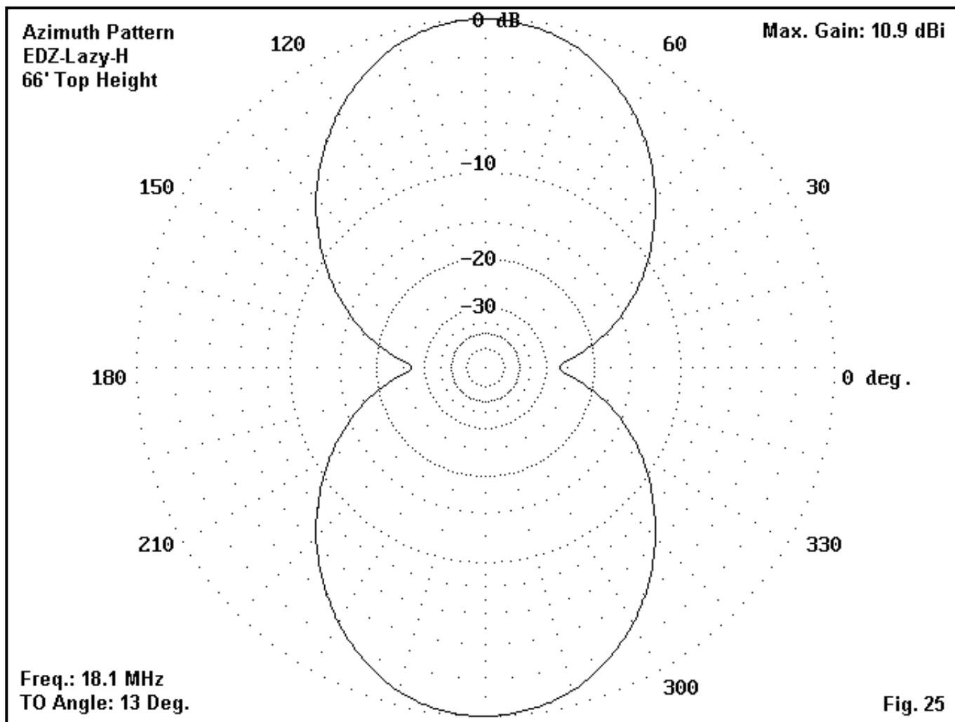
As we decrease frequency, the beamwidth will become wider and the EDZ "ears" will diminish. Below 12 meters, we obtain only a 2-lobe pattern. **Fig. 25** shows the pattern for 17 meters, where it is now wide enough to provide broad coverage. However, the nulls of the ends of the wires are greater than 25 dB down from the main lobe, making the antenna highly directional.
