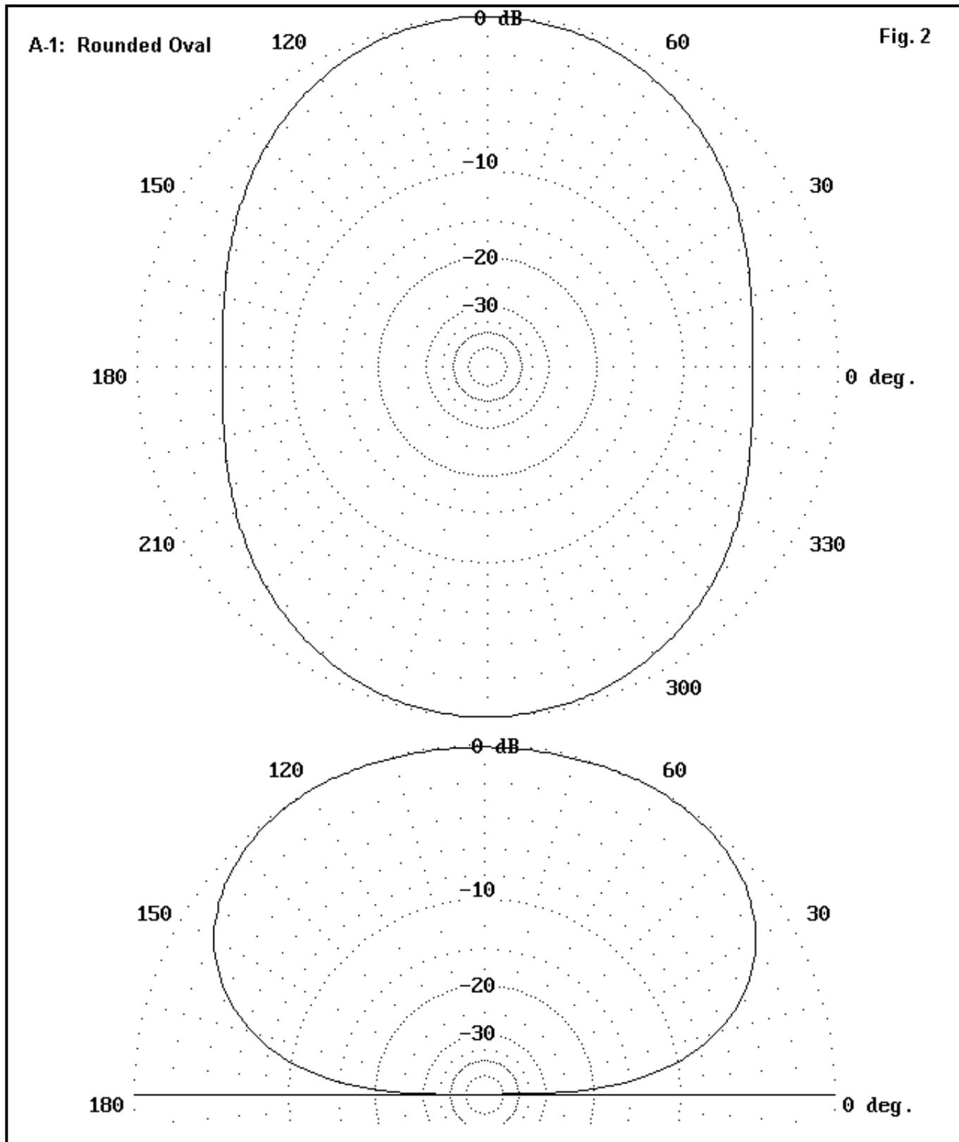
The oval azimuth pattern in **Fig. 2** is typical for horizontal wire antennas at heights under  $1/2$  wavelength ( $wl$ ). The lower the height, the more circular the pattern. As we increase the height, the radiation off the ends or edges of the antenna decreases. Gradually, the pattern becomes dimpled and fades into the next pattern type (A2).
