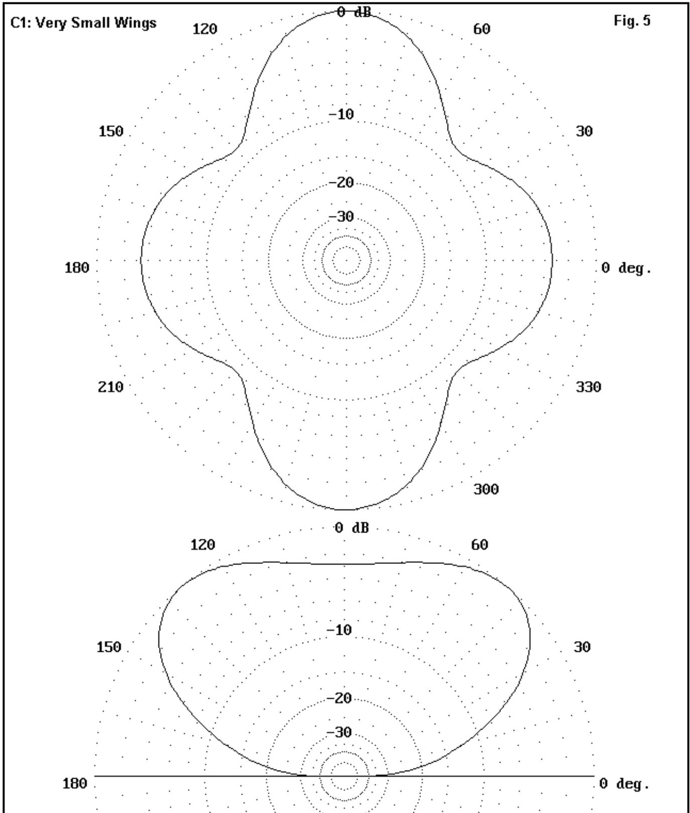
With VOHPL loops operated above their fundamental frequency, patterns do not always break up in the ways typical of doublets. We do not obtain cloverleaf or daisy-petal azimuth patterns. One of the variations for lobe formation (shown in **Fig. 5**) is the development of side "wings" off the edges of the antenna. In most cases, when these wings are small, antenna performance tends to be
