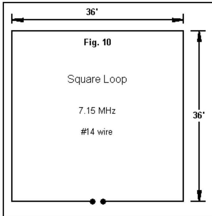
A square quad loop (**Fig. 10**) cut for approximate resonance on 40 meters at about 66' high places its lower wire at about the 30' level. The square shape makes this VOMBA among the most compact of those we have so far examined. Again, the change in length and orientation of the sides will give this version some distinct performance trends, compared to the deltas.
