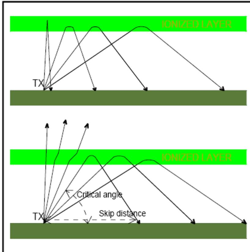
*Fig. 12.1. Simplified picture, only one layer is taken into account. The top sketch illustrates propagation with radio waves frequencies lower than the critical frequency; all the sky waves return back to the earth. The bottom sketch illustrates propagation with radio waves frequencies higher than the critical frequency.*
