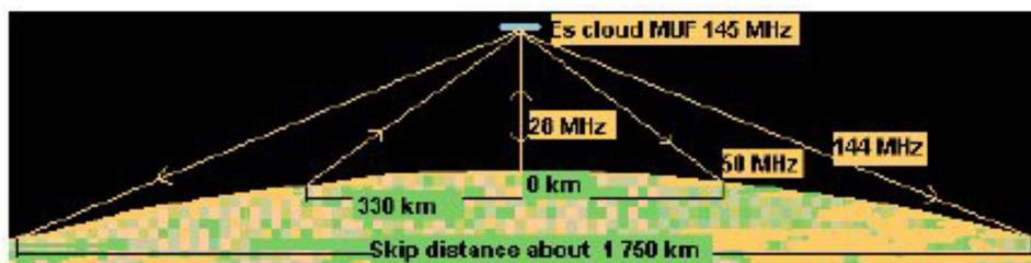
*Fig. 23.1. Illustrates the minimum skip distance of the 10-, 6- and 2 meters band with an Es cloud having a MUF of 145 MHz. With such a cloud overhead or nearby, you are able to make the closest 10-meter contacts right into your neighborhood.*
