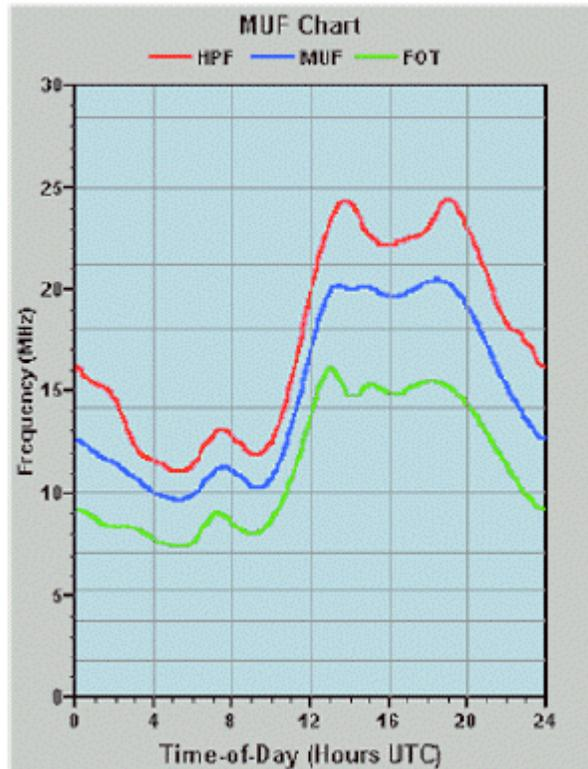
The determination of values for the MUF and related numbers requires a calculating engine (or a cadre of graduate students) to produce hourly projections along various paths. VOACAP (where the VOA part means Voice of America) has long been a standard for calculating a wide variety of propagation phenomena, both as an overall view and in detail. The program can calculate potential hops between points, with an indication of the MRM or most reliable mode.
