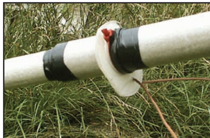
Figure 8 — Here is our polycarbonate element attachment plate: do not use a loop of wire at the corners to reinforce the elements. The loops can detune the elements.
