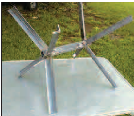
Figure 4 — The spider hub immediately after welding.
