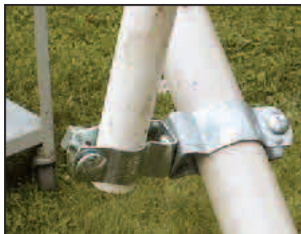
Figure 7 — The arm-to-brace connectors used in the prototype quad.
