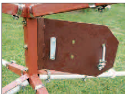
Figure 6 — The assembled hub and mast plate, with a coat of protective primer.
