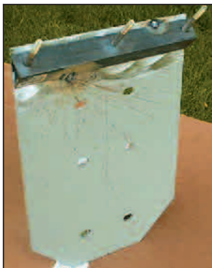
Figure 5 — The boom to mast plate attachment: note the 45° angle at the top of the plate and its bolts. This is used to attach the spider hub to the mast plate.
