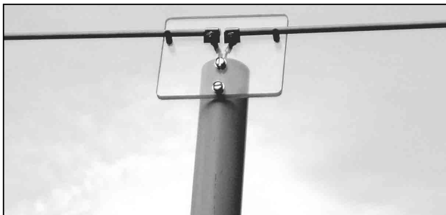
Photo B—A close-up of the center plate with a thin rod element clamped in place and supported by the outer posts.
